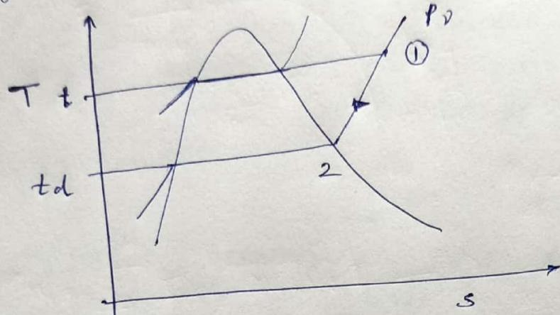
The temperature of air (dry bulb temp) and w.v is  $t$  and w.v. exists in superheated condition at ① its partial pressure is  $P_v$ . If the ~~is~~ air is cooled at constant pressure, its temperature will continuously decrease, and it will reach saturation temp  $t_d$ . At this point 2, w.v. will change phase from vapor to liquid. and first drop of water vapor (Dew) will appear. Hence this is called dew point temp
