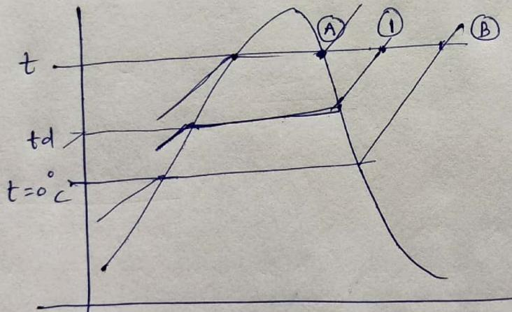
At the low partial pressure of water vapor  $h = f(t)$  only. Water vapor exists at point 1 and points A and B are at same temp
