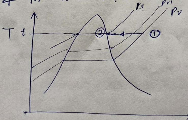
Water vapor in moist air is <sup>s</sup> superheated state ① and its temp is  $t$  (dpt) and partial pressure is  $P_V$ . If more moisture is added to this moist air keeping temp  $t$  constant, its partial pressure will continuously increase say  $P_{V1}, P_{V2}$  etc. until it reaches  $P_s$  at point ②. After this point 2
